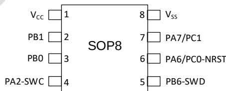
图 3-3 SOP8 Pinout1 PY32F002BL15S6-C (Top view)
